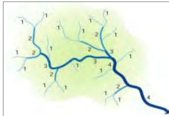
Small streams and tributaries play a significant role in overall river health. First-order (1) headwater streams combine to create larger second-order (2) streams and so on. (Image: United States Department of Agriculture)
