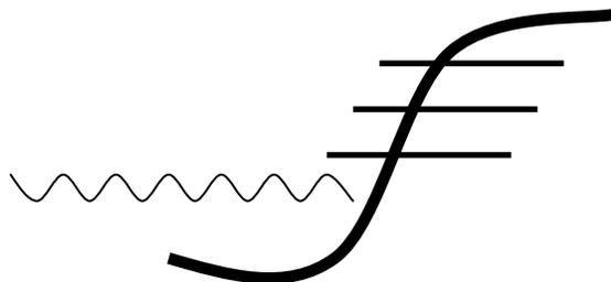
4. Measure the height of the erosion pins on the day they are installed (“Day 0” data) and again at periodic intervals, to the nearest millimeter.
